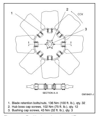
Figure 3-12 Fan Hardware Location and Torque
